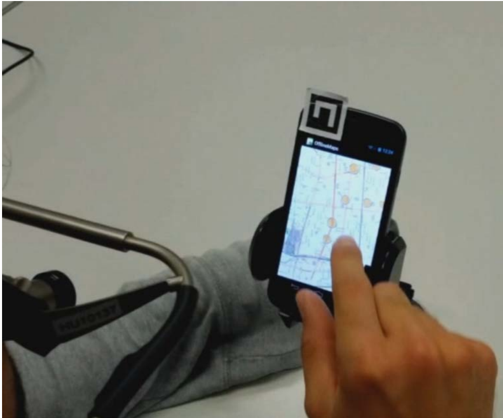
Figure 5: Study setup for gaze-based interaction with an interactive mobile map (refer to Giannopoulos et al., 2012). The user's gaze on the map during the interaction is recorded (in map coordinates), aggregated, and visualized when the user zooms out (circles). These circles are called GeoGazemarks and serve as visual bookmarks on the map.
